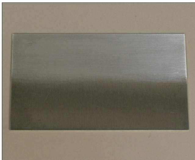
A-2 Aluminum oxide protects aluminum from corroding.
