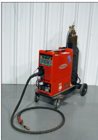
F-3 Aluminum-specific machines may have pre-programmed aluminum settings.
