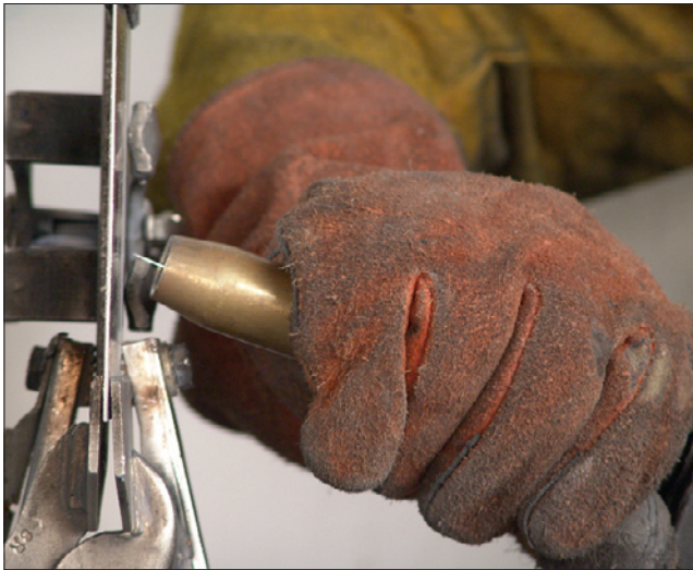
B-4 Nozzle-to-workpiece distance should be about 10–16 mm ( \frac{3}{8} – \frac{5}{8} ”).
