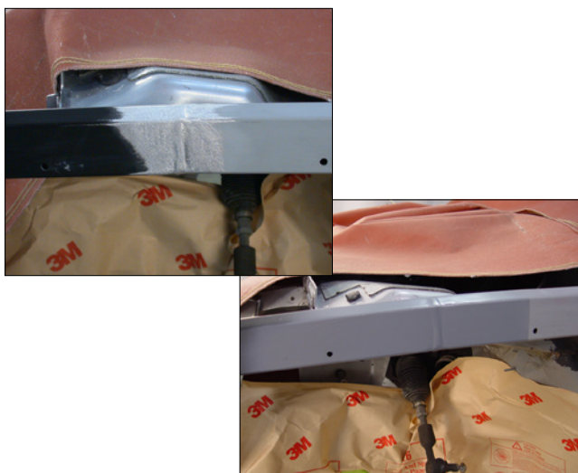
F-12 Epoxy primer is commonly used to coat bare aluminum.
