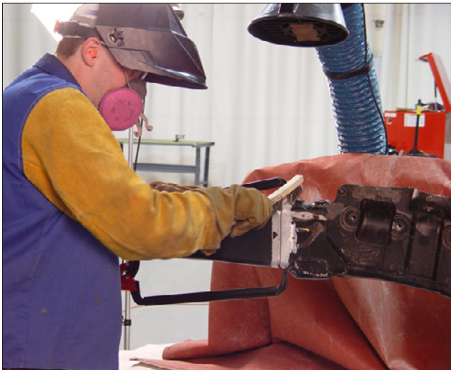
A-6 Weld as soon as possible following cleaning and part fit-up.
