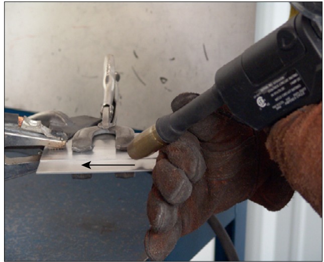
B-1 The welding gun is pointed and pushed away from the weld puddle.
