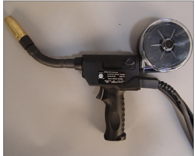
D-1 Spool guns may have flexible ends to increase accessibility.
