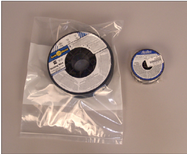
C-3 Electrode wire should be stored properly when not in use.
