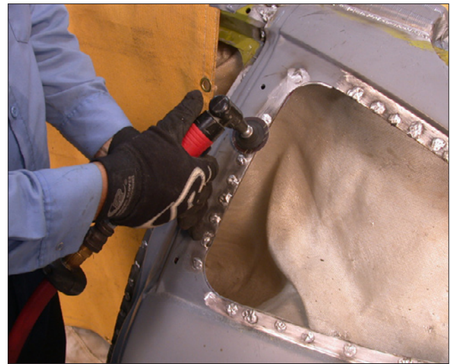
F-11 Grind welds where they will interfere with adjacent panel fit-up.
