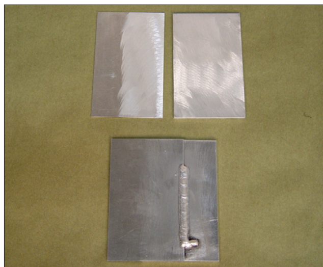
C-1 The AWQT fillet weld uses two coupons that are different thicknesses.
