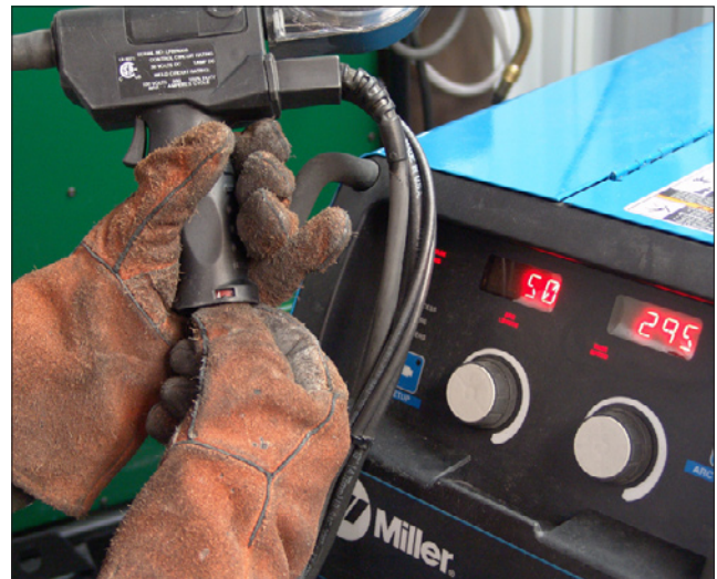
C-2 Increasing or decreasing amperage affects the heat of the weld.
