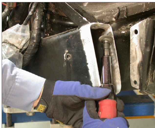
A-3 Every area of the weld joint must have coatings and oxide removed.
